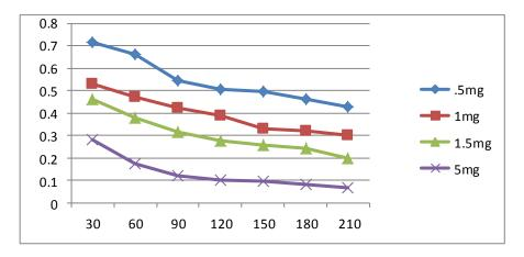
Figure 3: Rate of degradation of MB solution (1x10<sup>-5</sup>mol/L) with different amount of NMs.
