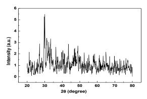
Figure 1: XRD pattern of nanoparticles from the roasted processed Camellia sinensis leaves
