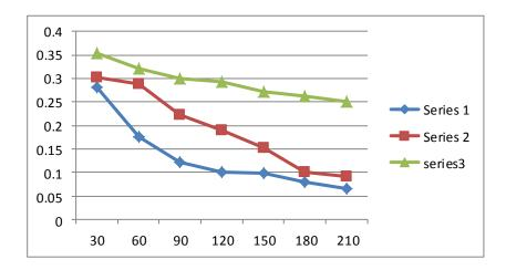
Figure 2: Action of NMs on different concentration of MB solution Series1- 1x10<sup>-5</sup>mol/L, Series2-5x10<sup>-5</sup>mol/L, Series3-1x10<sup>-4</sup>mol/L
